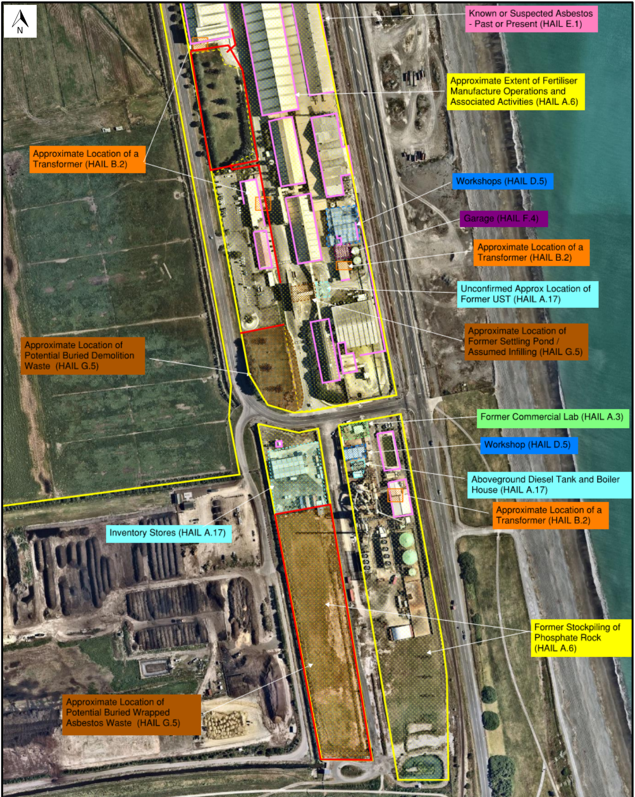
Figure 5: HAIL Activities Identified During the PSI on/in the Vicinity of the Site
