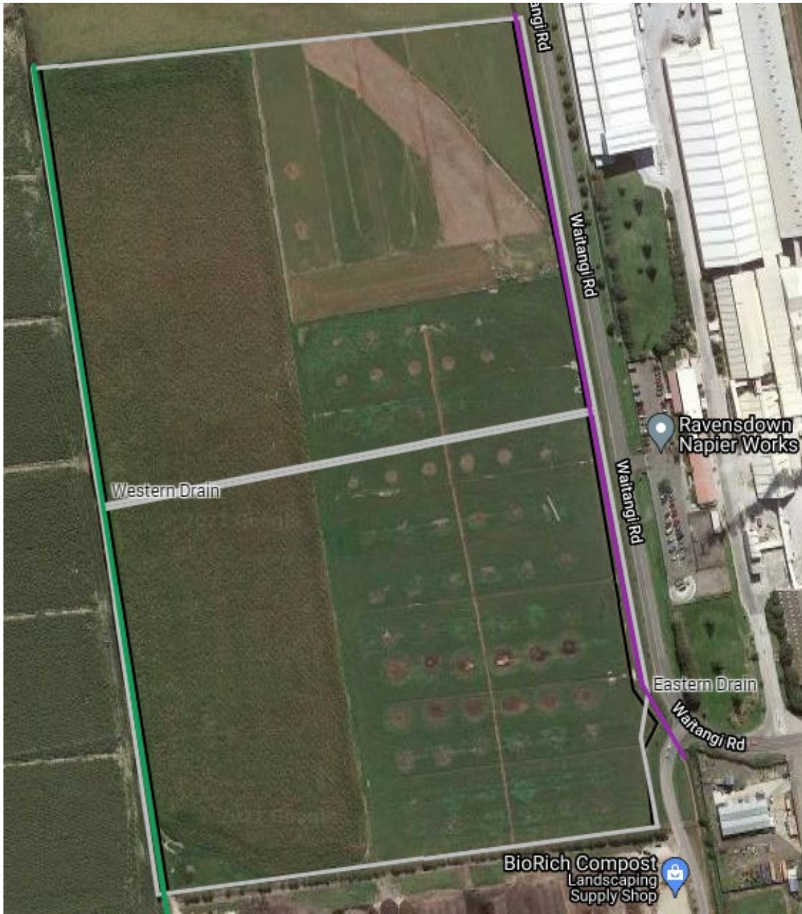
Figure 2: base image of Cadastral boundaries and location of drains on western and eastern boundaries
