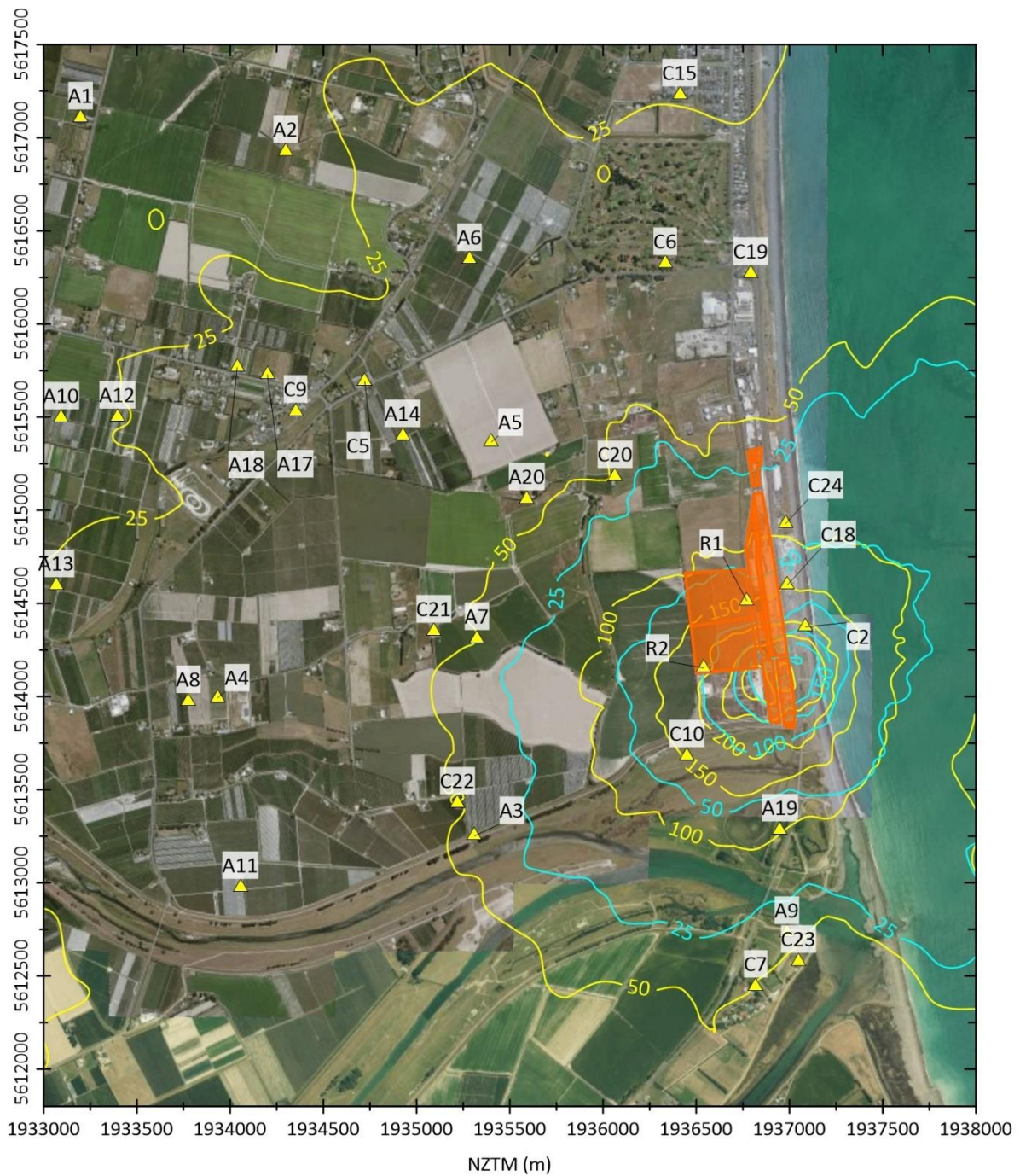
Figure 12.1: Comparison of predicted maximum 1-hour average \text{SO}_2 concentrations associated with the Acid Plant discharging at its maximum emission rate of 60 kg/hr (yellow contours) with conditions that give rise to lower velocity, temperature and emission rates (3 m/s, 50 °C, 20 kg/hr – blue contours).
