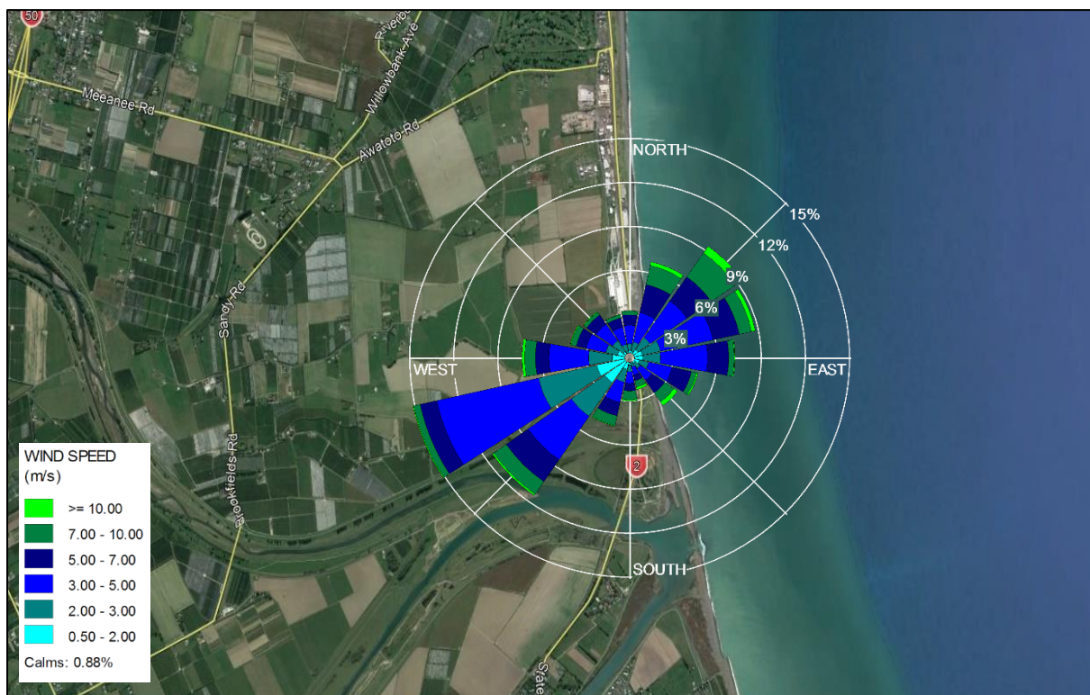
Figure 4.3: Wind rose for the Ravensdown Napier site generated from the measured site data used in the CALMET data set.
